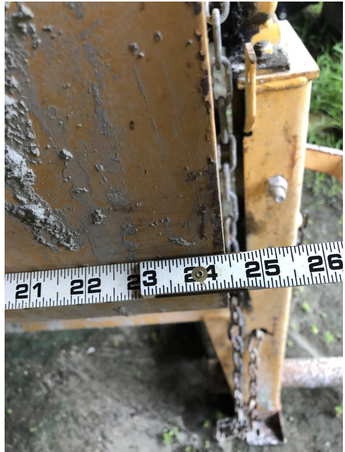
Figure 6C - Measure Drum Length in inches. ( 24-1/2 Inches on this mixer)
