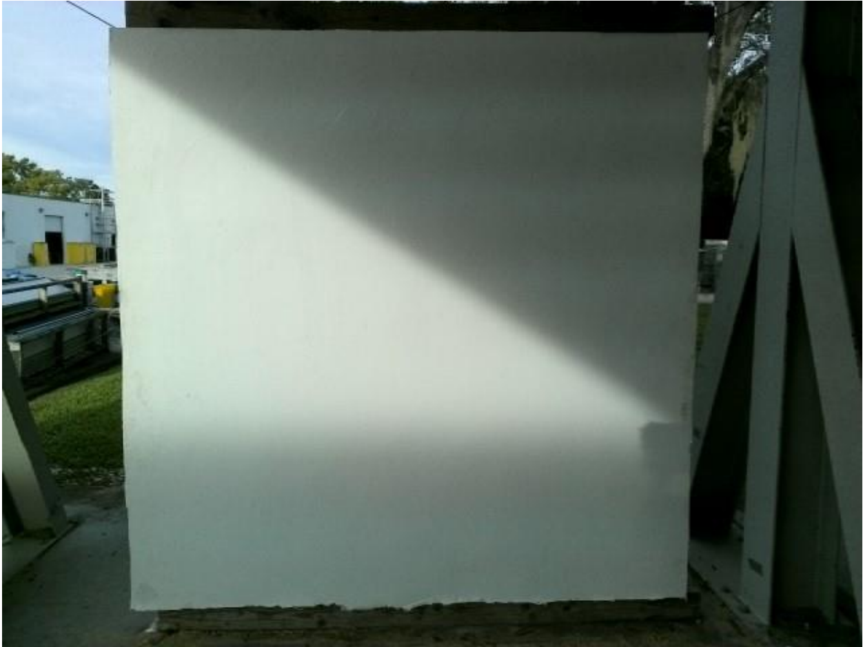
Test specimen after Transverse and Racking Loads
